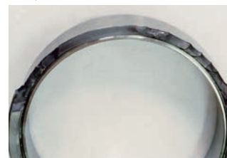
Inner ring cracking
