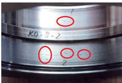
Brinelling on raceway surface of outer ring
