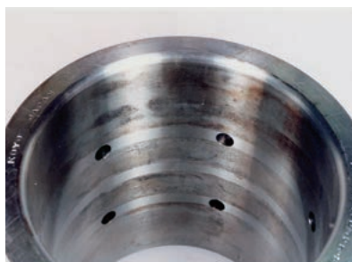
Fretting on bore surface of inner ring
